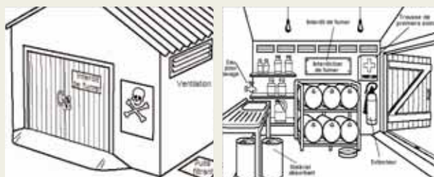
Figure 3 & 4: Large store for pesticides - internal and external view.
