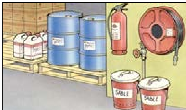
The products are not placed directly on the floor. The safety equipment (see sand in buckets and fire control systems) has been installed.
