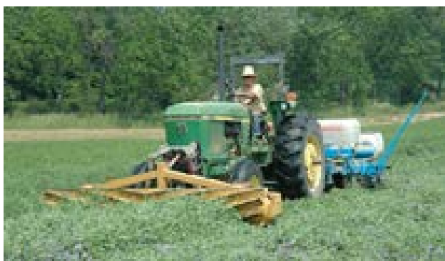
Rolling and seeding the vetch in one pass
