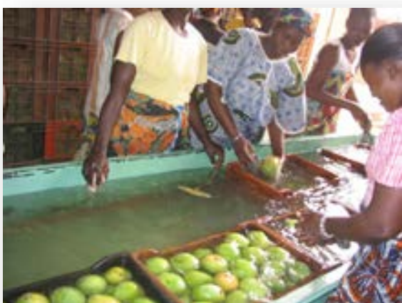
Basin for washing mangoes by immersion (Photo B. Samb)
