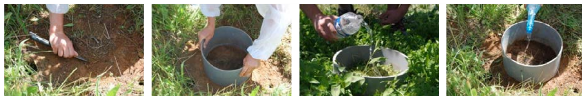
Figure 7 - Clear the surface; insert a cylinder; pour in a quantity of water; record the time it takes to soak into the soil Source: Lhote, technical meeting, Ctif/ITAB
