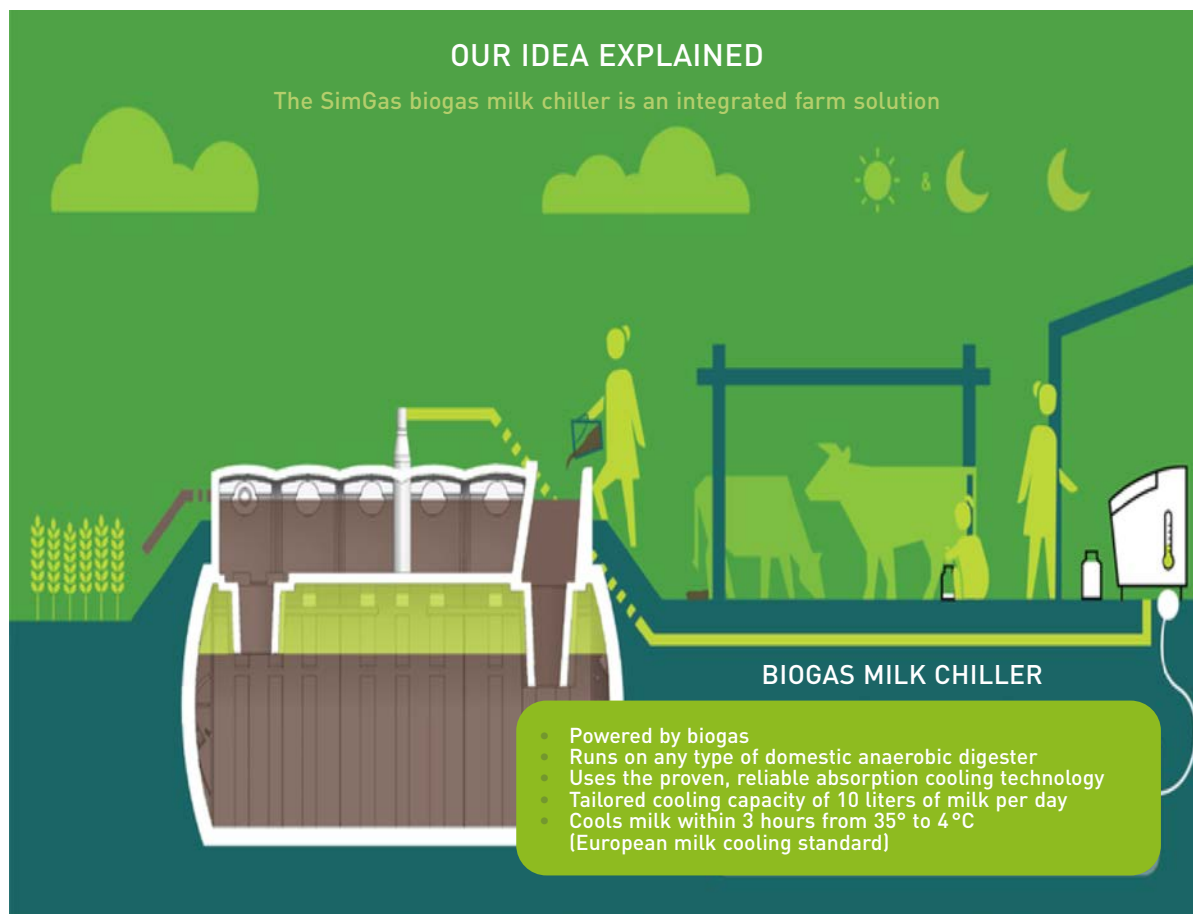
Figure 25 - Biogas refrigeration [Source https://challenges.openideo.com/challenge/agricultural-innovation/improve/biogas-powered-milk-chiller-for-small-scale-dairy-farmers-in-eastern-africa/comments ]
