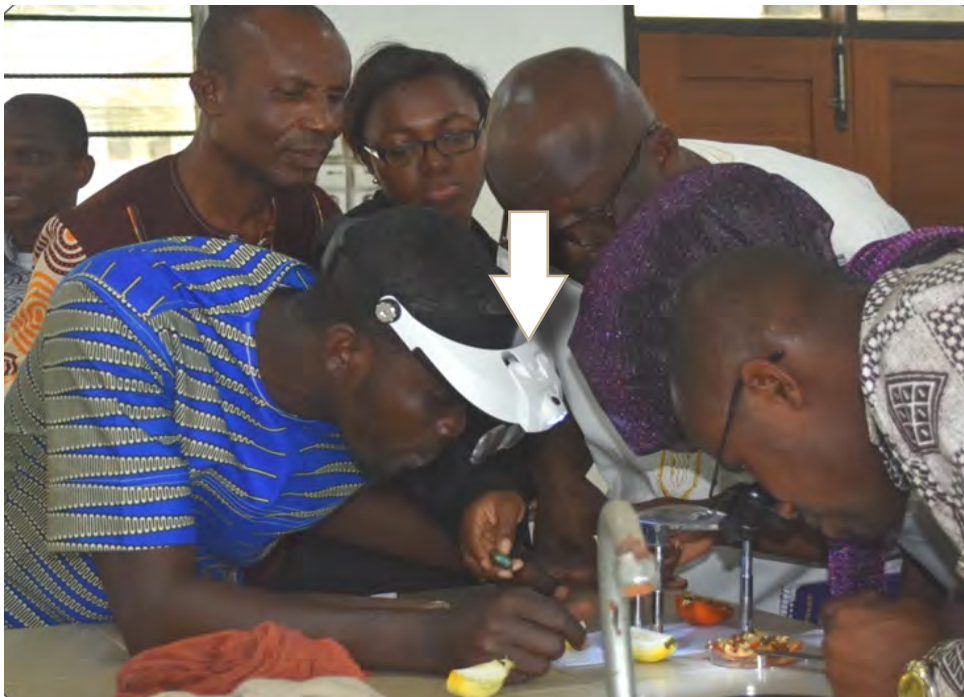
Figure 13: Using the head visor, fitted with a magnifying lens, for inspecting the presence of quarantine pest in produce. (Photo by KO Fening, University of Ghana) (see arrow).
