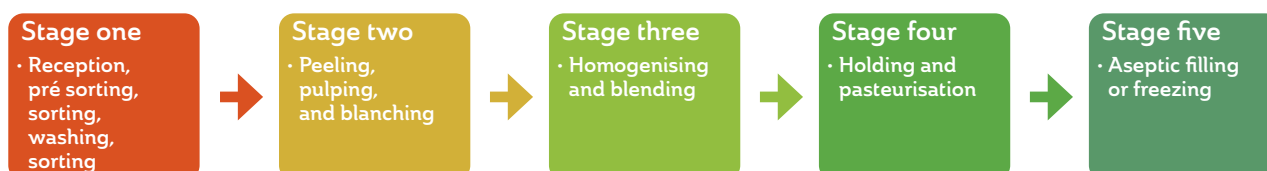
Figure 6. Production stages of sweet potato puree
