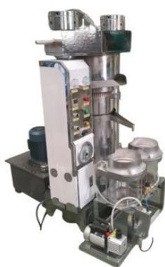
A hydraulic press is a machine that generates a compressive force. The pressure throughout the closed system is constant. One part of the system is a piston acting as a pump, with a modest mechanical force acting on a small cross-sectional area; the other part is a piston with a larger area that generates a correspondingly large mechanical force.
