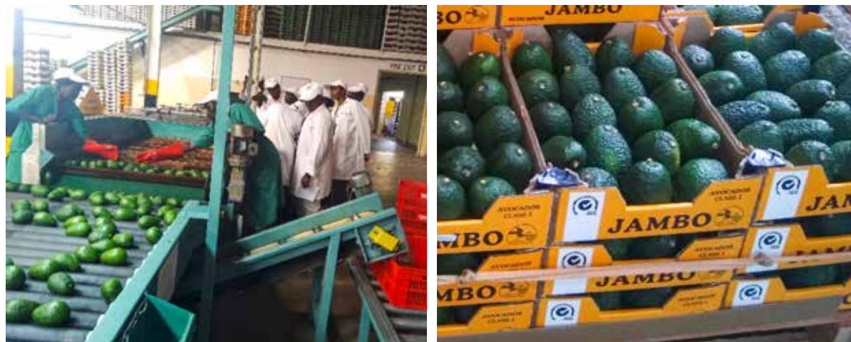
Figure 112 — Fruits sorted using machine in the pack house (left) and graded according to variety, size and same maturity stage
