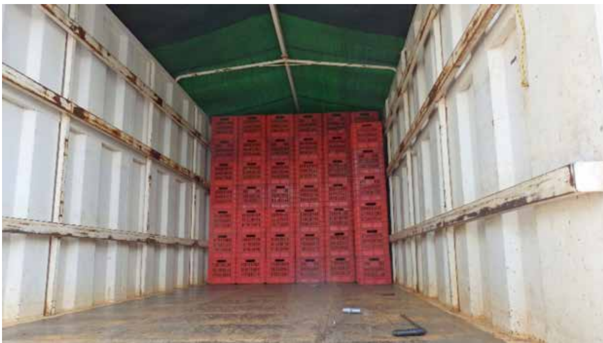
Figure 110 — The correct way of transporting avocado fruits from field to pack house in crates and stacked onto each other in a truck
