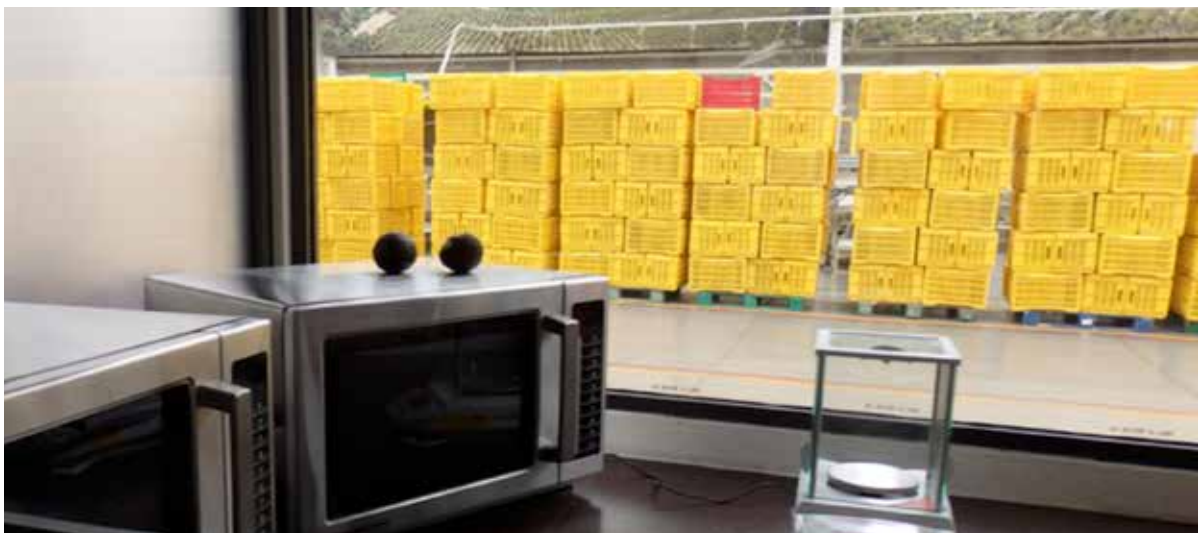
Figure 102 — Simple apparatus (Microwave and a digital weighing scale) used to determine maturing level of fruits using dry matter content method
