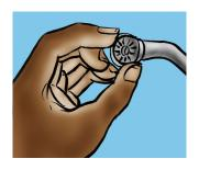
Choose the nozzle, that will give the required flow rate and droplet size.
