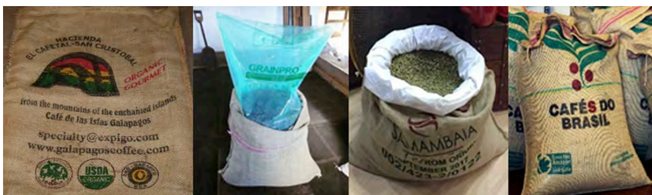
Figure 16: Left: Ecuadorian jute 60 kg bag of organic certified coffee. Source: Galapagocoffee.com. Right: Jute 60 kg bags of organic certified coffee and bags with Grainpro liner. Source: Grainpro.com.
