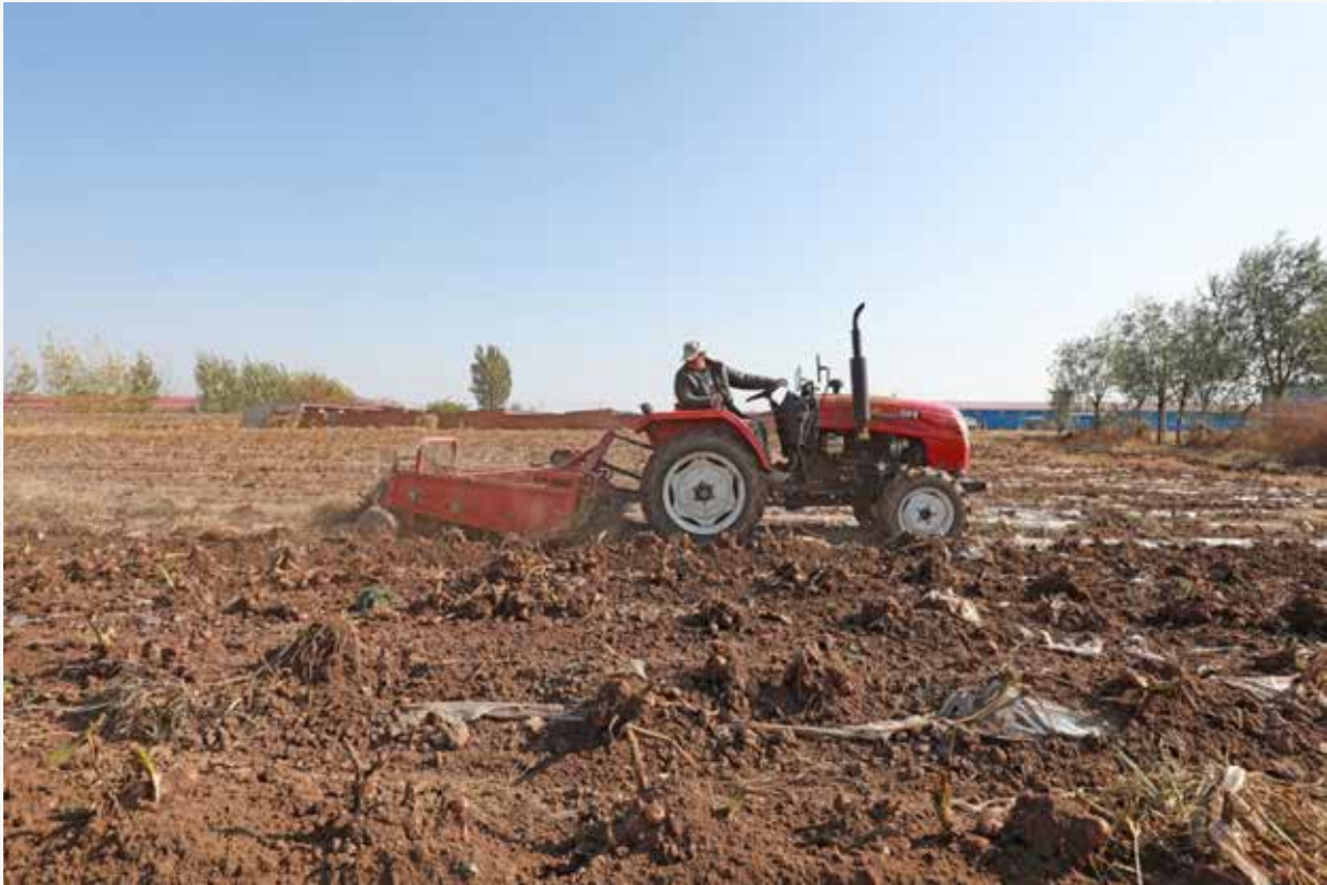
Figure 104 — Mechanised harvesting of eddoe taro with a lifter that leaves the cormels on the surface, from Hebei Province, China Photo: https://fr.123 #ID 187058142
