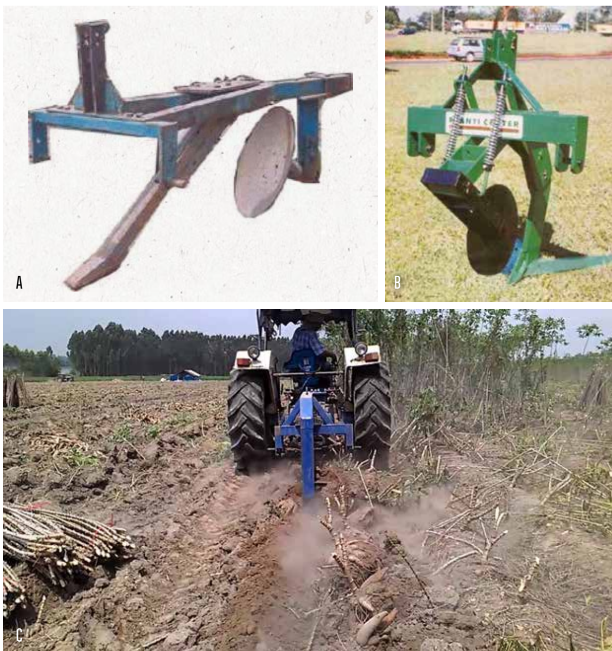
Figure 122 — Showing tractor-operated semi-mechanised harvesters: (A) NCAM-harvester made in Nigeria; (B) CLAYUCA-harvester model P600 made in Brazil, and (C) a semi-mechanised cassava harvester mounted on a tractor
