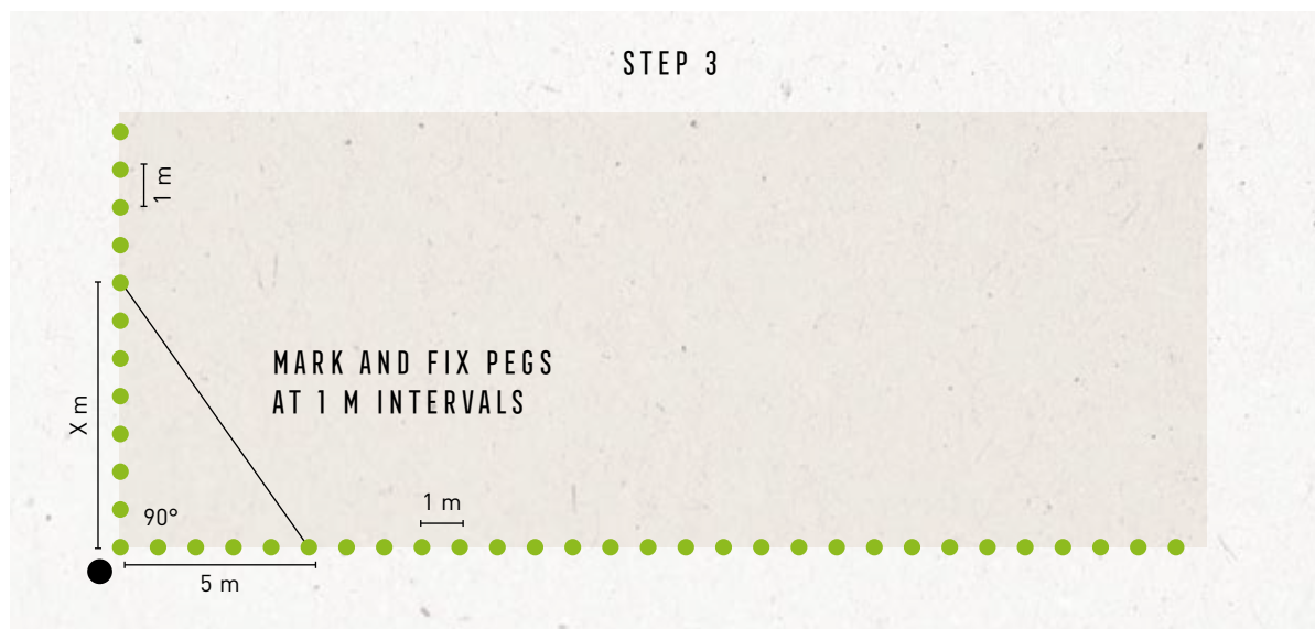
Figure 49 — Showing step 3 in marking a plot
