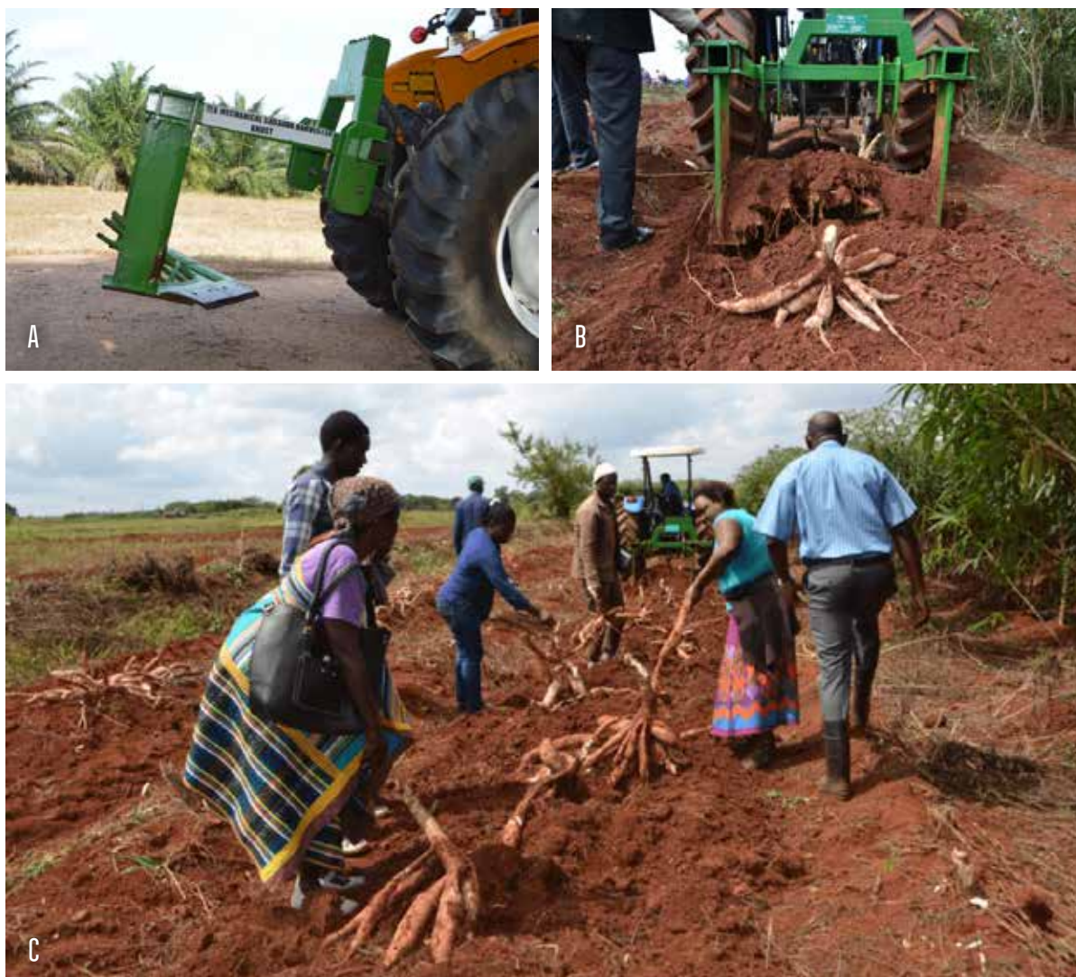
Figure 123 — Showing (A) a fully mechanised TEK cassava harvester mounted on a tractor; (B) the TEK harvester in use in the field and (C) farmers manually collecting cassava tubers dug up by the TEK mechanical harvester
