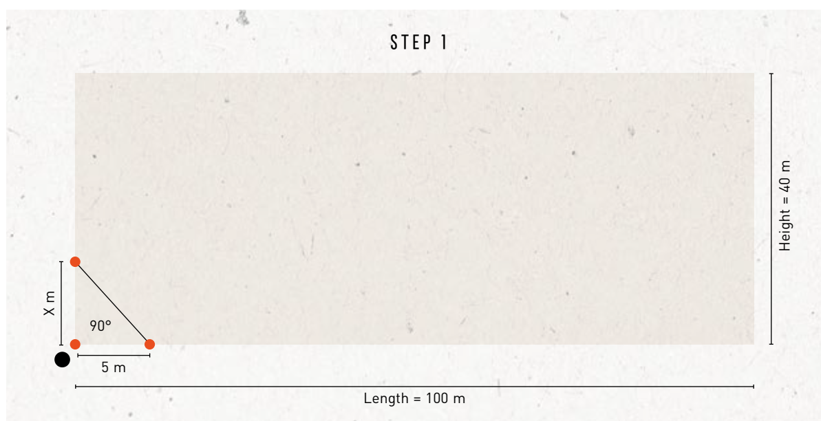
Figure 47 — Showing step 1 in marking a plot
