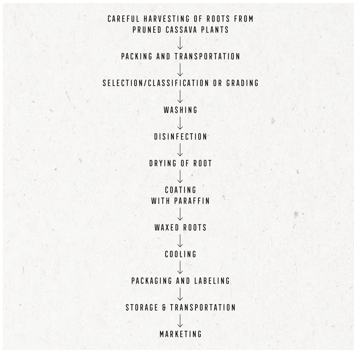
Figure 133 — Showing the essential packhouse operations carried out during waxing cassava with paraffin wax Source: Adopted from Matovu et al. (2016)
