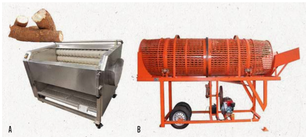
Figure 135 — Showing cassava (A) peeling & washing machine (all in one) and (B) peeling (alone) Source: https://www.juiceprocessline.com/wp-content/uploads/2021/02/cassava-washing-and-peeling-machine.jpg ; https://nationaltoday.com/wp-content/uploads/2020/06/Tapioca-640x514.jpg
