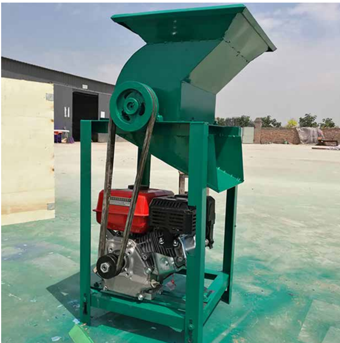
Figure 138 — Showing a grating machine used for grating cassava Source: https://sc04.alicdn.com/kf/HTB1rpKjKaSWBuNjSsrBq6y0mVXaa.jpg
