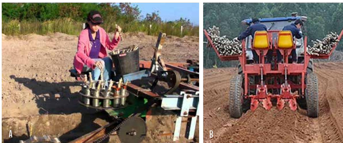
Figure 54 — Showing mechanised two models (A & B) of cassava planters mounted on tractors
