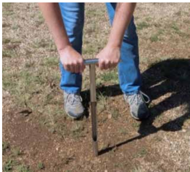
Figure 19 Example of a stainless steel soil sampler to assess soil quality of target fields, 7(Penn Ltd)
