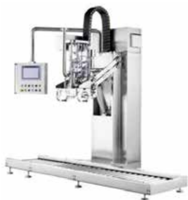
Figure 12: Aseptic filler. Source: Tropical Food Machinery
