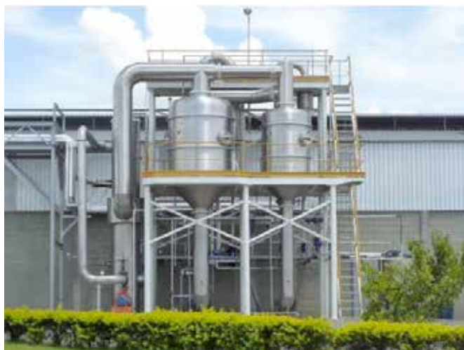
Figure 11: Forced circulation evaporator. Source: Tropical Foods.
