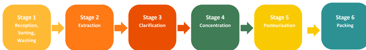
Figure 9: Typical citrus juice processing stages
